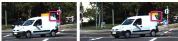
Figure 1. A car moving against a varying background. Nearly half of the patch centered on a Harris corner at the object boundary is part of the background.
